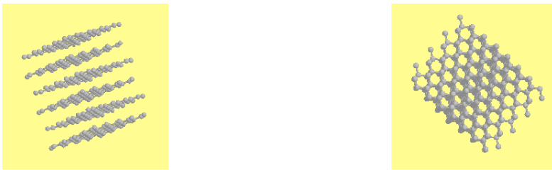
FIG. 1: On the left, the graphite lattice has a preferred slicing, contrary to the diamond lattice on the right [16].
